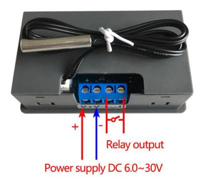
Note:It is a relay output mode and cannot be used as a power module. It cannot output voltage. The load needs to be connected to a separate power supply.
