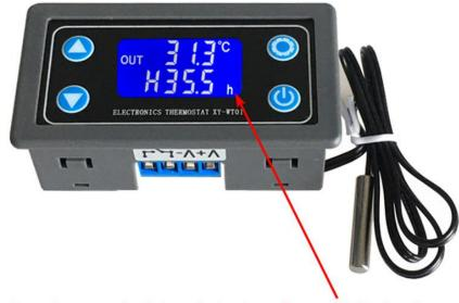
When the OPA is delayed, the interface will display 'h'.
